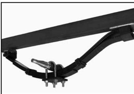
Figure A: Standard Axle Installation
