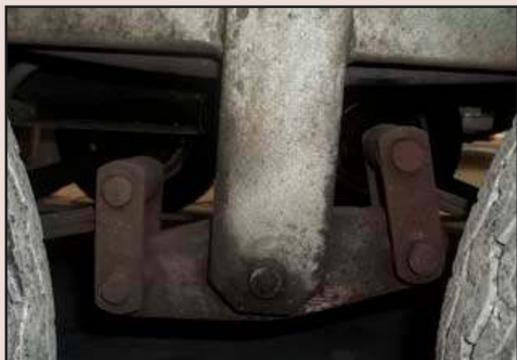
In relation to maintenance the shackle pins and bushes can often require replacement within 15-20,000km (not good is it!) We recommend replacing springs at 70-80,000km as after this point they become very prone to breaking. Sometimes money is better spent (once these systems need some significant maintenance) converting to the Rocker-Roller system. The Rocker-Roller is not an independent system, but a cost effective step-up from a Rocker system.
