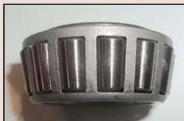
periodic use and cannot be heard from the tow vehicle when badly worn, plus on tandems endure a severe load on every corner. As an example a typical 16' caravan often has 'Falcon' front end wheel bearings supporting a load of around 1500kg. A Falcon has 4 wheels supporting virtually the same weight, so it's no surprise these caravan bearings show earlier signs of wear!
